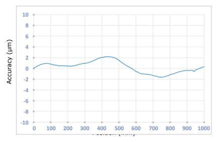
Accuracy graph: deviation between the value measured by the encoder and the value measured by the reference system.
