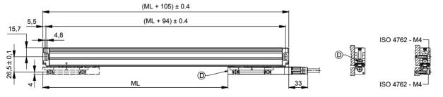
ML = Measuring length, P = Machine guide, C = Measuring length start, ML (20 mm absolute), D = Compressed air inlet M5, Dimensions in mm
