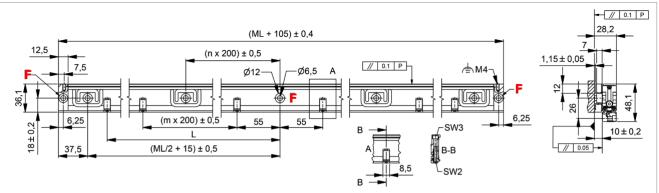
The supporting bar fixing determines the position of the FEP. Use the fixing hole  $\mathbf{F}$  (central or lateral) that makes the FEPs of the scale and its supporting bar coherent.
