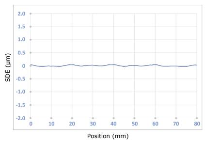
SDE (sub-division error) graph: accuracy of the interpolation device within the single grating pitch.
