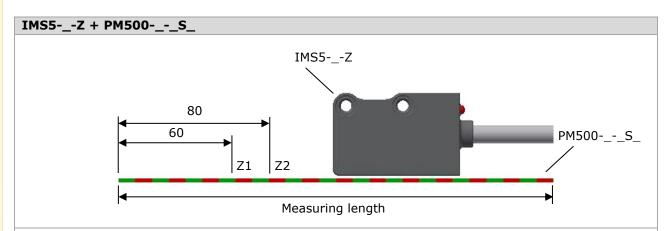
Example: Magnetic scale type PM500-\_-\_S\_ with reference index at 60 mm and 80 mm (from the left).
