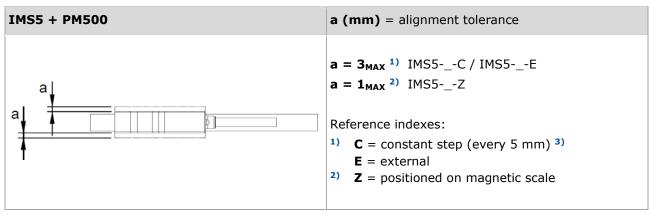
With 100  $\mu$ m resolution, the constant step is 10 mm.
