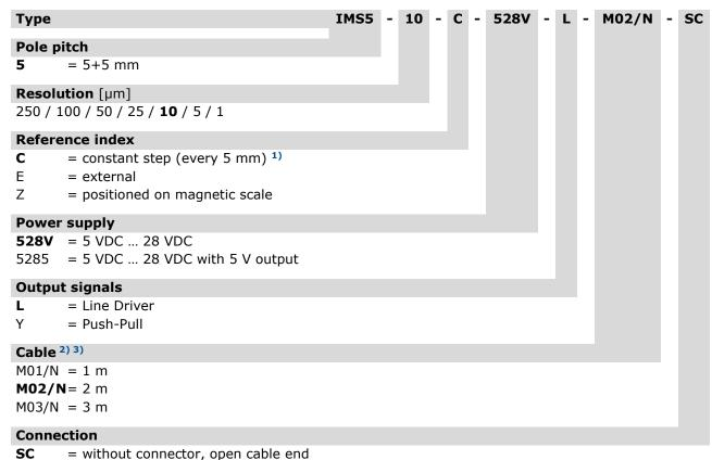
With 100 µm resolution, the constant step is 10 mm.
